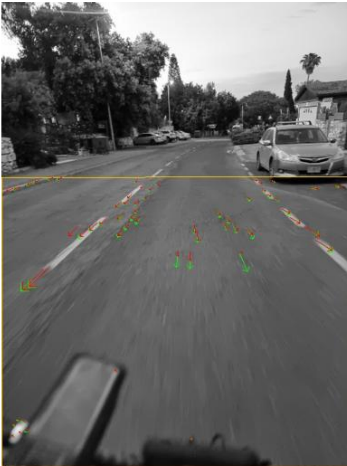
Figure 7.5: A rear-camera frame during a validation ride, showing the amber ground-plane sampling region and per-point optical-flow arrows (green: template-matching reference; red: production KLT).
